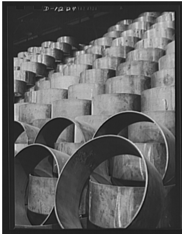
Fig. 10. Alfred T. Palmer, Tank manufacture (Chrysler) . Stockpiles such as these need constant replenishment now that M-3 tanks have reached a mass production schedule. These are wheel suspension lever forgings, stored outside the huge Chrysler tank arsenal in Detroit where 10,000 workers are turning out 28 ton rolling arsenals for the Army, 1942 ©Library of Congress
