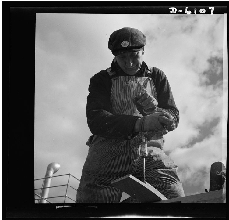
Fig. 5. Howard Liberman, Production. Submarine chasers. Shipwrights preserve many hand skills. Brace and bit are needed to fit coamings to machine gun wings just aft of the wheelhouse of a wooden subchaser under construction in an Eastern boatyard. Marine Construction Company, Stamford, Connecticut, mars 1942 ©Library of Congress
